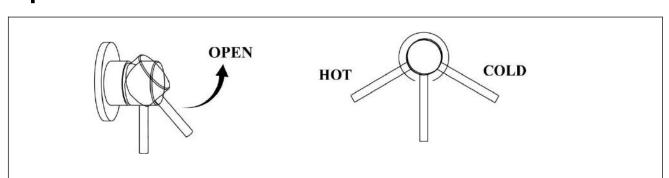
By lifting the Lever Handle upwards, the valve will be activated. Water flow will increase by continuing to lift up the Lever Handle. By rotating the Lever Handle counter-clockwise, the water temperature will decrease. By rotating the Lever Handle colockwise, the water temperature will increase.
